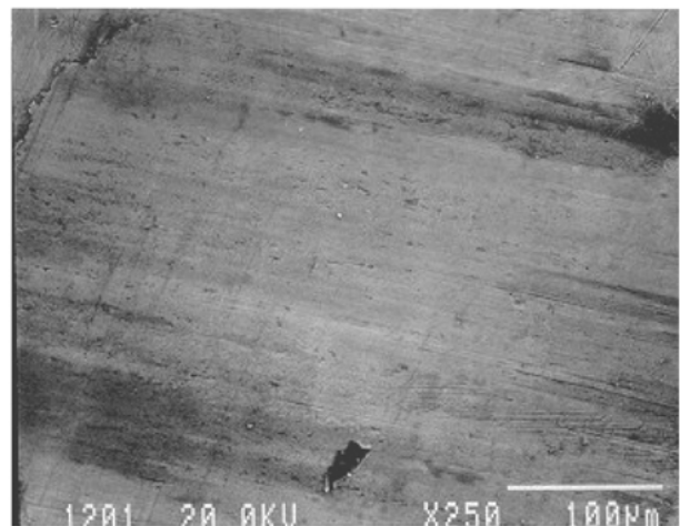
Figure 7 SEM micrograph from worn area of Ti-6Al-4V pin after testing under dry conditions (RH 50%) against a DLC coated Co-Cr-Mo disc.
